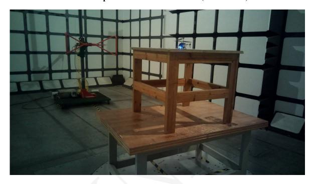
**Radiated Spurious Emissions Test View (Above 1GHz)**
