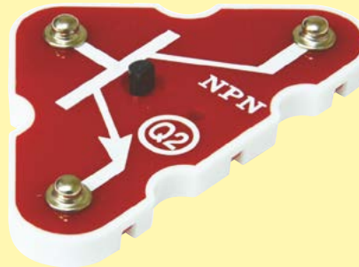
NPN transistor (Q2)
