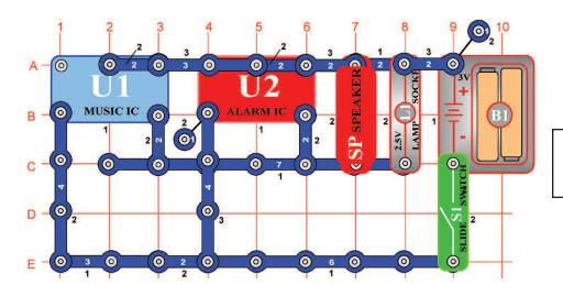
In the circuit, the outputs from the alarm (U2) and music (U1) IC's are connected together. The sounds from both IC's are played at the same time.
