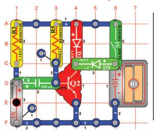
Turn the slide switch (S1) on. There will be only a weak light emitting from the green LED (D2). By blowing on the mic (X1) or putting it near a radio or TV set, the green LED will emit light, and its brightness changes as the loudness changes.
