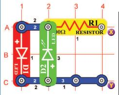
Use this circuit to check the polarity of a battery. Connect your battery to X & Y on the drawing using the jumper cables (your 3V battery pack (B1) can also be snapped on directly instead). If the positive (+) side of your battery is connected to X, then the red LED (D1) will be on, if the negative (-) side is connected to X then the green LED (D2) will be on.
