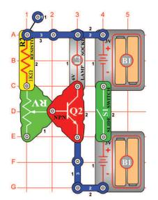
OBJECTIVE: To compare transistor circuits.
