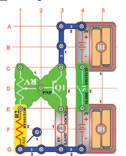
OBJECTIVE: To demonstrate adjusting the gain of a transistor circuit.
