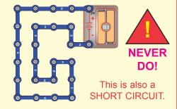
When the slide switch (S1) is turned on, this large circuit has a SHORT CIRCUIT path (as shown by the arrows). The short circuit prevents any other portions of the circuit from ever working.
