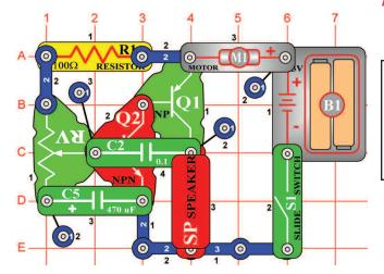
Build the circuit on the left and place the fan onto the motor (M1). Turn on the slide switch (S1) and move the setting on the adjustable resistor (RV) across its range. You hear screaming sounds and the fan spins.
