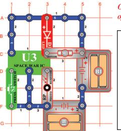
OBJECTIVE: To vary the speed of a fan activated by light.
