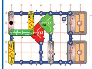
Install the parts. The lamp (L2) will be on. It will be off as long as you blow on the mic (X1). Speaking loud into the mic will change the brightness of the lamp.
