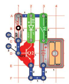
OBJECTIVE: To compare transistor circuits.
