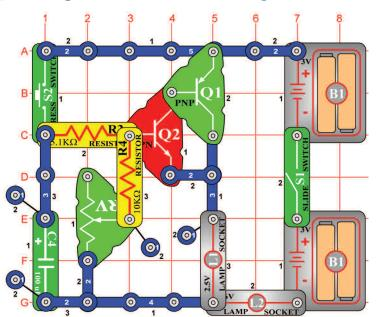
OBJECTIVE: To build a lamp that stays on for a while.
