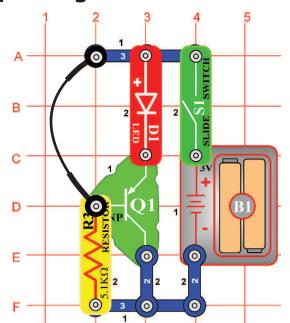
OBJECTIVE: To build a transistor light alarm.
